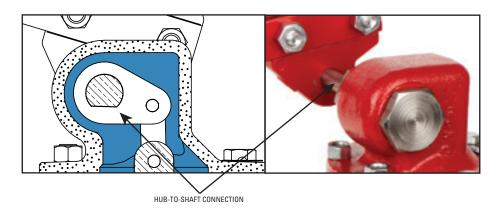
We have quickly corrected this issue by tightening the tolerances (making the shaft dimensions larger).
