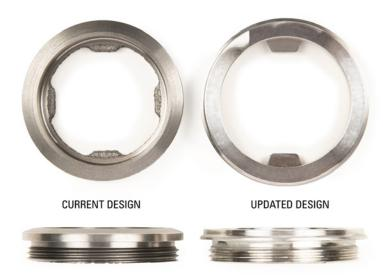
The current full port seat has four internal "fins". The new seat will feature a slight design modification and only two "fins" in the inner diameter. This change is driven by continuous improvement efforts to enhance the flow capability for full port regulators and low pressure control valves.
