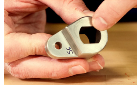
ORIGINAL HUB (KEYWAY) Prior to 10/2017
