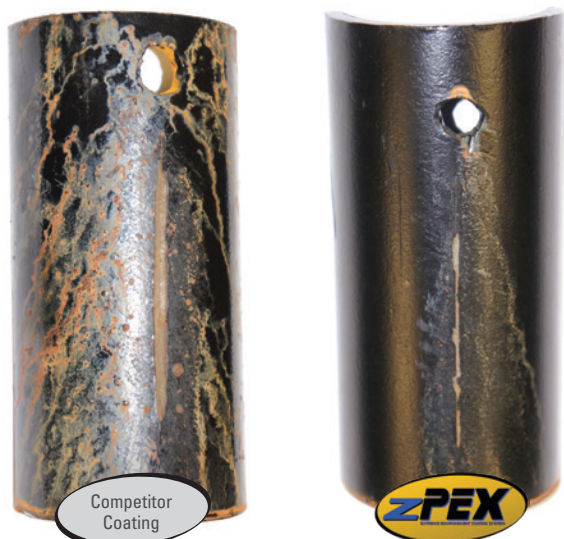
Material Loss, coating "creepback" and blistering
