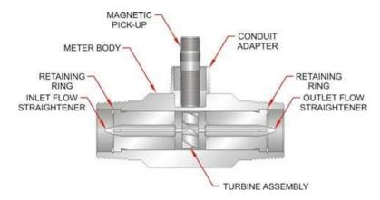
**NOTE:** If the meter repair kit part number ends in NCC (no calibration), it was not factory calibrated. For these repair kits, use the nominal K factor supplied.
