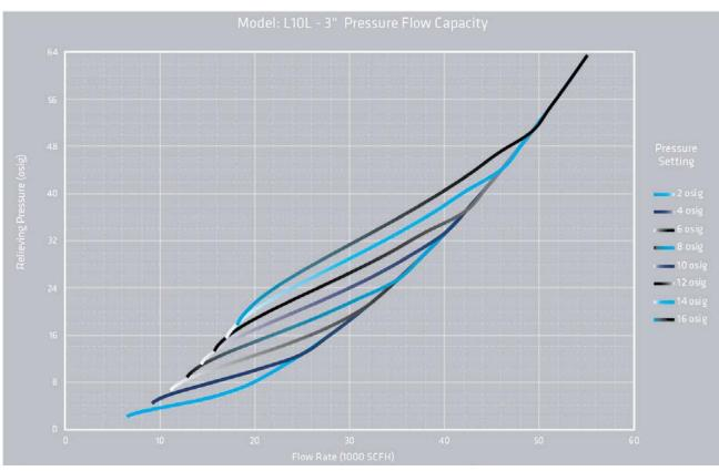
The test equipment, procedures, and reporting methods meet the requirements of standards API 2000/ISO 28300 and ISO 16852. The equipment, procedures, and methods have been reviewed and certified by TÜV SÜD. Flow data are for tank mounting or end of line and includes entrance loss, exit loss and internal losses. Flow values based on air at 60°F venting to atmospheric pressure of 14.6959 psia.
