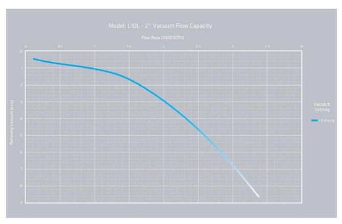
The test equipment, procedures, and reporting methods meet the requirements of standards API 2000/ISO 28300 and ISO 16852. The equipment, procedures, and methods have been reviewed and certified by TÜV SÜD. Flow data are for tank mounting or end of line and includes entrance loss, exit loss and internal losses. Flow values based on air at 60°F venting from atmospheric pressure of 14.6959 psia.
